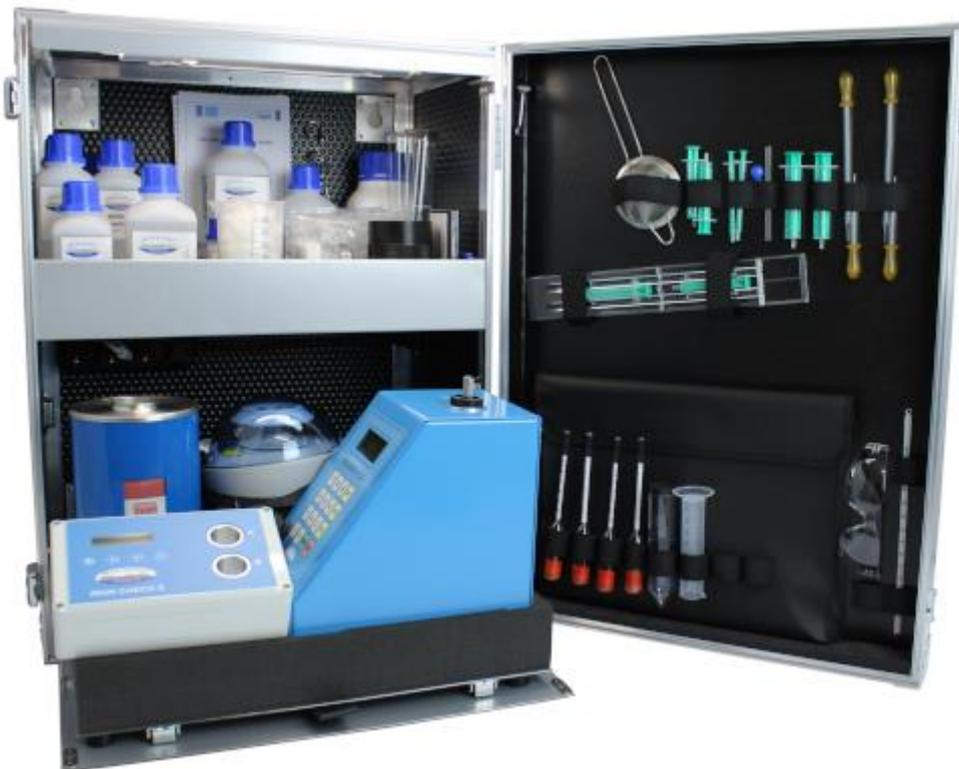
**BRENNSTOFF- UND SCHMIERÖL-TESTKABINETT Option II: MT CAT FINES CHECK + TOTAL IRON CHECK
