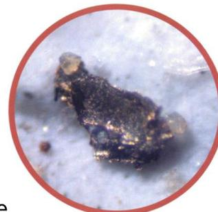
Particles of various nature (metal, rust etc.) can be found in the oil sample.
